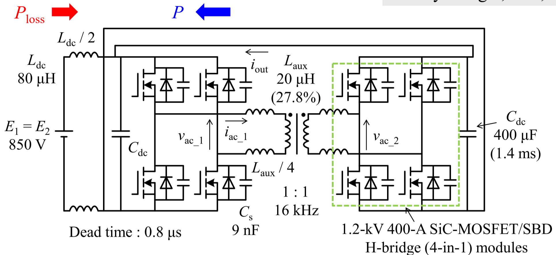
Conversion efficiency  $\eta = \frac{P}{P + P_{\text{loss}}}$  Tolerance : lower than 0.005%
